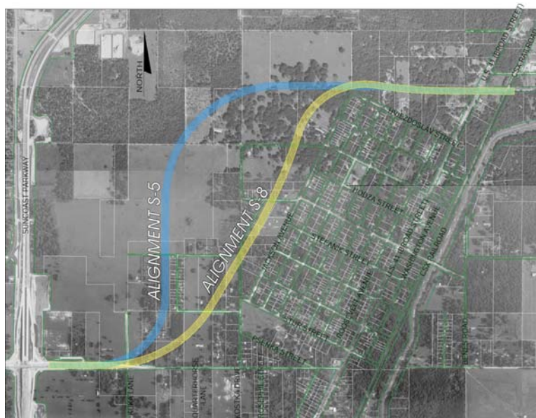
FIGURE 2-1 AYERS ROAD EXTENSION ALIGNMENTS
