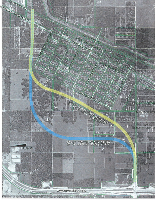
FIGURE 2 AYERS ROAD EXTENSION ALIGNMENTS
