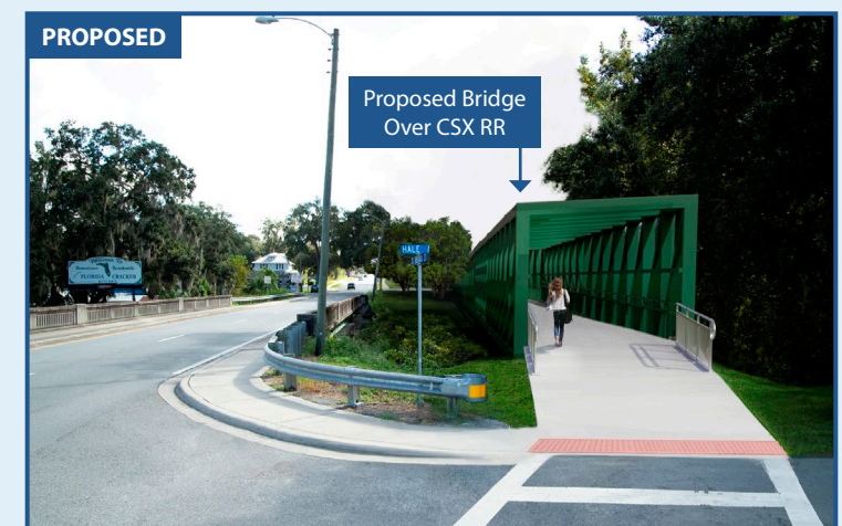
Broad Street at Hale Avenue - Looking East Prefabricated Steel Truss Option for Trail Bridge
