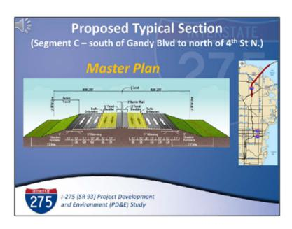
The Recommended Build Alternative for Segment C consists of providing tolled express lanes adjacent to the existing non-tolled travel lanes on I-275.
