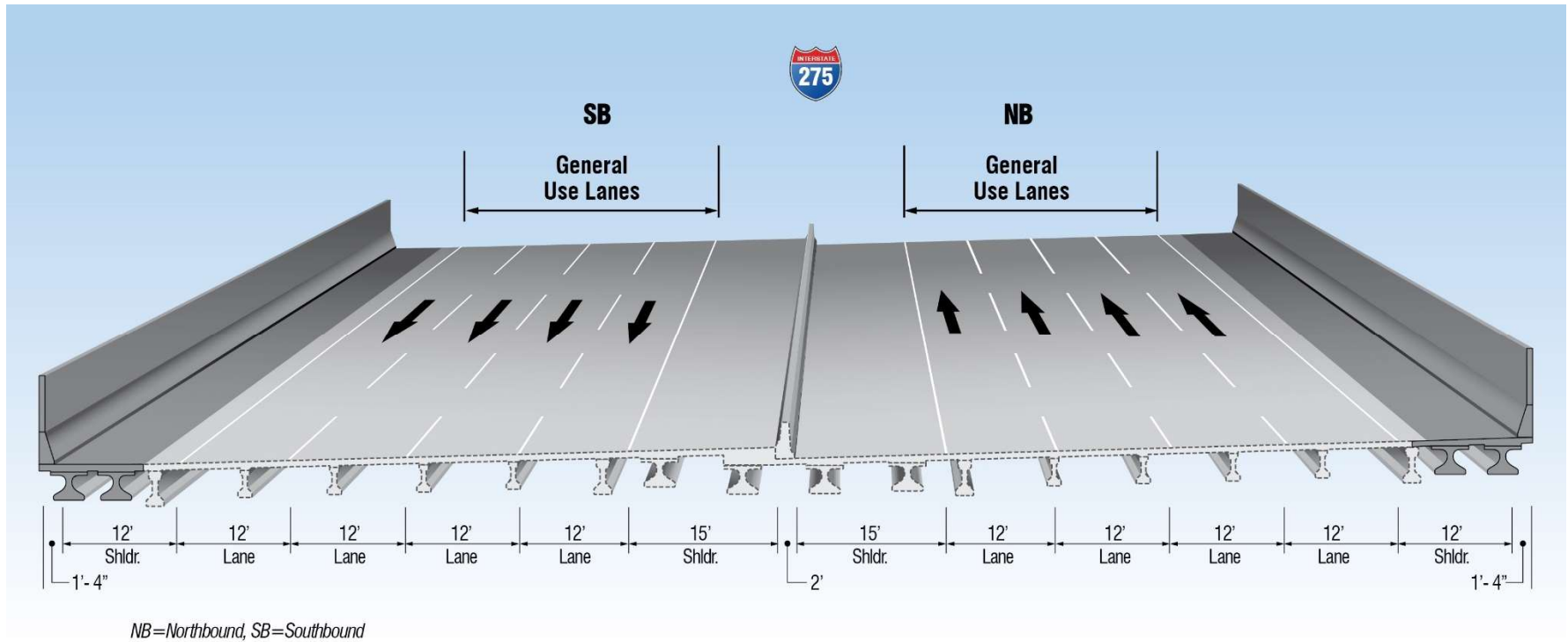
Figure 16: Proposed Bridge Typical Section
