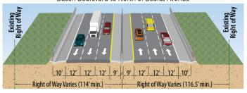
**Figure 2** shows the typical section for the Preferred Build Alternative.
