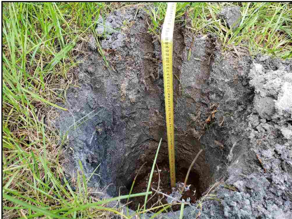
Photo 9. Typical soil stratigraphy of ponds located in an upland environment.
