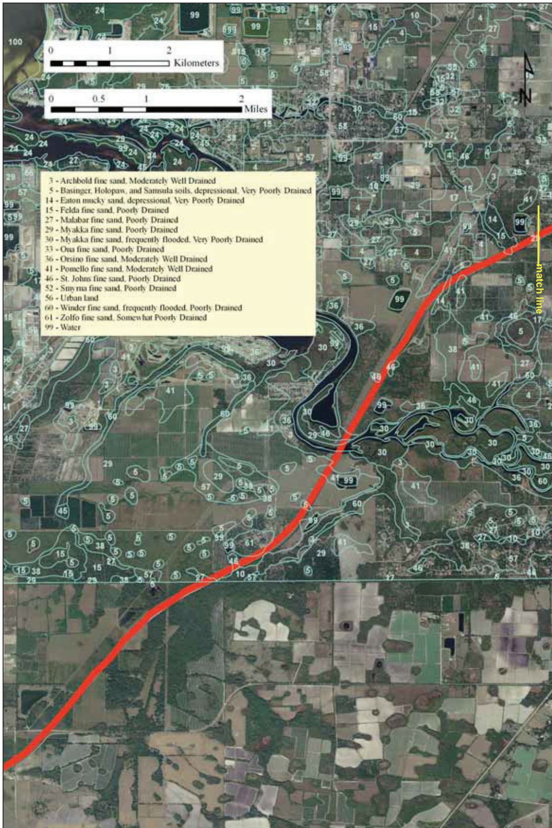
Figure 2-7 Soil types and their drainage characteristics along the I-75 PD&E Study corridor, Hillsborough County (USDA 2005a).
