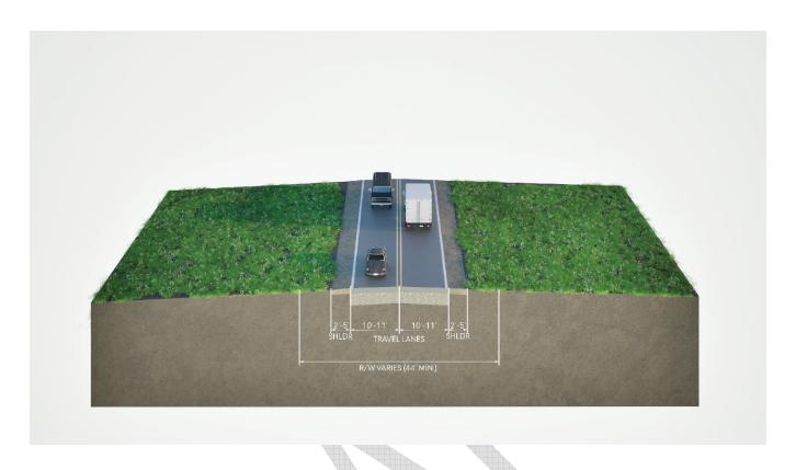
Figure 1-2: McIntosh Road Existing Typical Section
