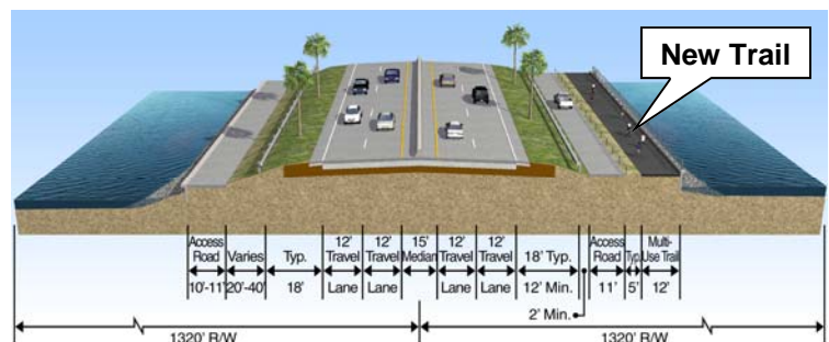
Proposed Roadway/Trail Typical Section 3
