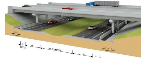
Typical Section 2 - is a suburban roadway with two 11-foot travel lanes and a seven-foot buffered bike lane in each direction. This typical section complies with the FDOT minimum 45 mph design speed but would require a design variation if the roadway is expanded to six lanes in the future.
