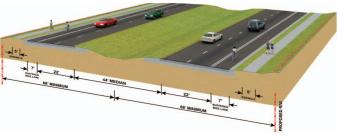
**Typical Section 1** - is a suburban roadway with two 11-foot travel lanes and a seven-foot buffered bike lane in each direction. This typical section requires a minimum of 136 feet of right-of-way and complies with the FDOT minimum 45 mph design speed.
