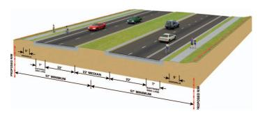
**Typical Section 4** - is an urban roadway with two 11-foot travel lanes and a seven-foot buffered bike lane in each direction. This typical section requires a minimum of 114 feet of right-of-way and complies with the FDOT minimum 45 mph design speed.
