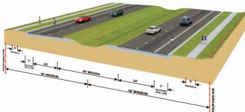
**Typical Section 5 -** is a high speed suburban roadway with two 12-foot travel lanes, a five-foot sidewalk, and a seven-foot buffered bike lane in each direction. The travel lanes are separated by a 40-foot median with eight-foot inside shoulders with a 50 mph design speed.
