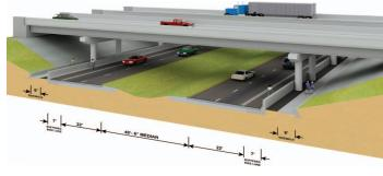
**Typical Section 2** - is a suburban roadway with two 11-foot travel lanes and a seven-foot buffered bike lane in each direction. This typical section complies with the FDOT minimum 45 mph design speed but would require a design variation if the roadway is expanded to six lanes in the future.
