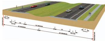
**Typical Section 3** - is a high speed suburban roadway with two 12-foot travel lanes and a seven-foot buffered bike lane in each direction. This typical section requires a minimum of 160 feet of right-of-way and complies with the FDOT minimum 50 mph design speed.
