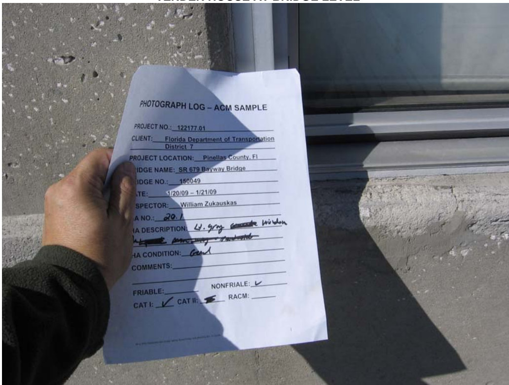
PHOTO 50 – 01/21/09 – SAMPLE 20.1 – HA 20 GRAY CAULK TENDER HOUSE EXTERIOR AND INTERIOR OF METAL WINDOW FRAMES
