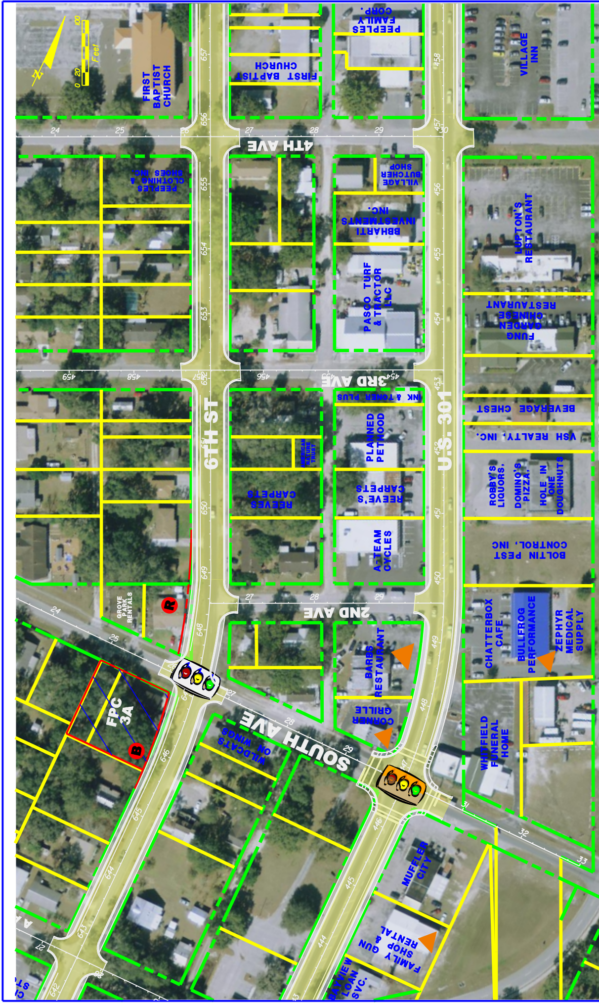
ALIGNMENT AND RIGHT OF WAY 6TH STREET AND US 301(GALL BLVD.) ONE-WAY PAIR ALTERNATIVE
