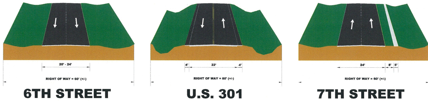
EXISTING TYPICAL SECTIONS
