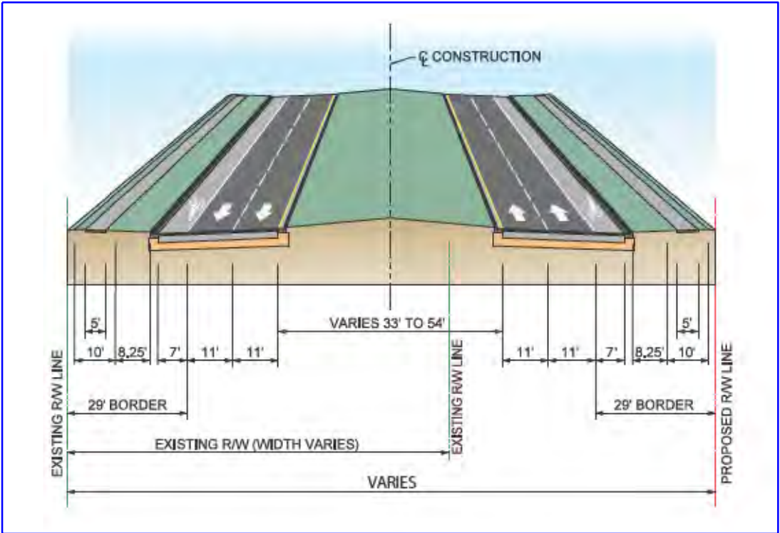
PROPOSED URBAN TYPICAL SECTION CHANCEY ROAD TO SOUTH OF SR 39 (BUCHMAN HIGHWAY) 45 MPH DESIGN SPEED
