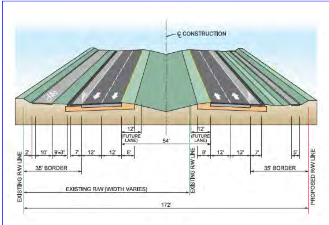
PROPOSED SUBURBAN TYPICAL SECTION SOUTH OF PROPOSED SR 56 TO CHANCEY ROAD 50 MPH DESIGN SPEED
