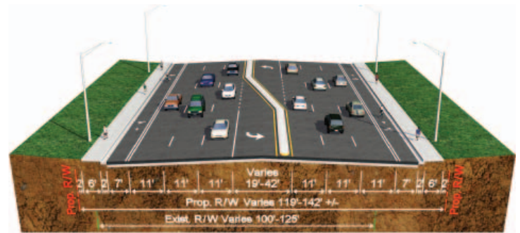
Proposed Typical Section from Palm Avenue to Gibsonton Drive (Proposed typical section from Gibsonton Drive to Lula Street is very similar to this one)
