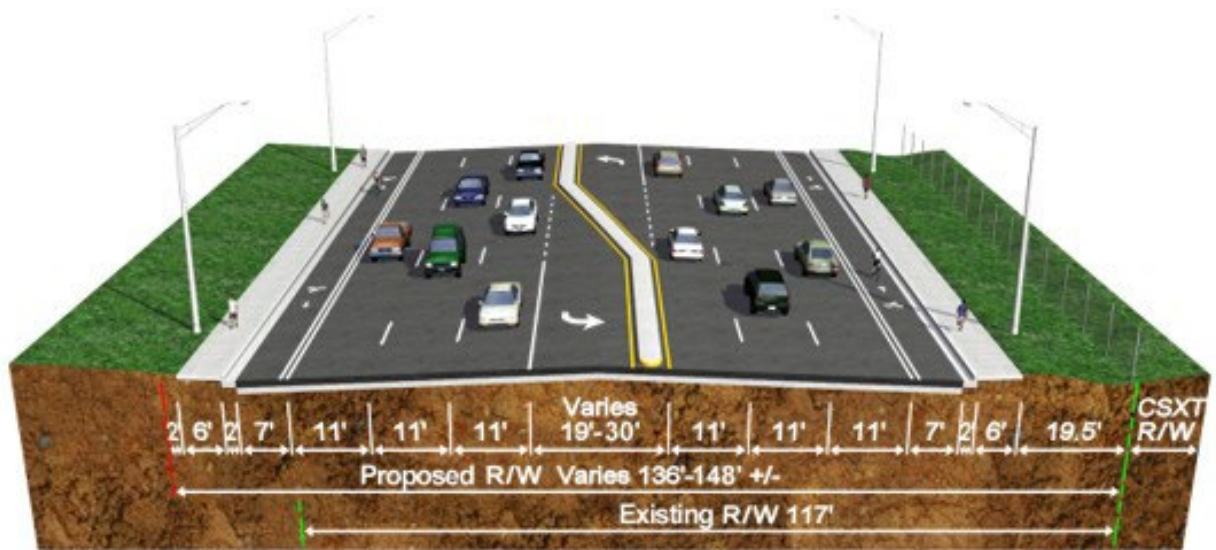
Figure 1-6 | Proposed US 41 Roadway Typical Section - Gibsonton Drive to Lula Street
