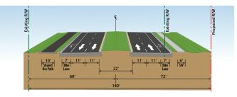
At the Hillsborough River and Old Lakeland Highway/CSX Railroad locations, the bridges will be replaced with twin bridges with two 12-foot travel lanes with 6-foot inside shoulders and 10-foot outside shoulders. Both bridges will include barrier separated 10-foot walkway to accommodate future shared use path and/or sidewalk (bicycle and pedestrian) accommodations and will be located within the existing 160-foot ROW. (See image below)
