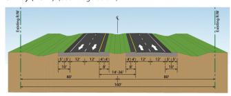
From north of Townsend Road to Cindy Lane, the roadway consists of a suburban typical section with two 12-foot travel lanes in each direction located within a proposed 245-foot wide ROW and includes a 6-foot sidewalk on the east side of the road and a 12-foot shared use path on the west side of the road. (See image below)
