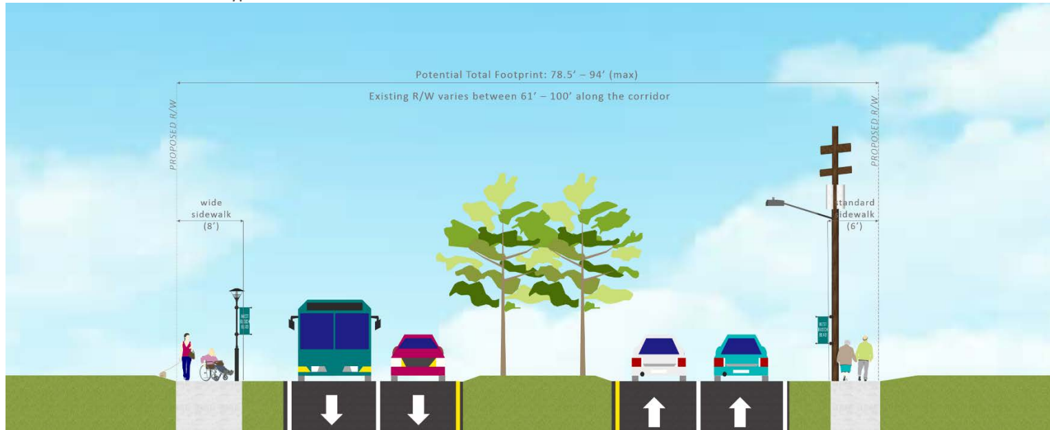
Exhibit 30. 4-Lane Alternative Typical Section
