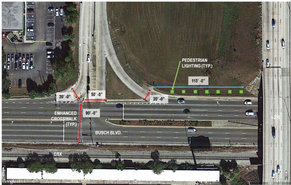
ENHANCED CROSSWALKS AND PEDESTRIAN LIGHTING AT BUSCH BLVD. (WEST)
