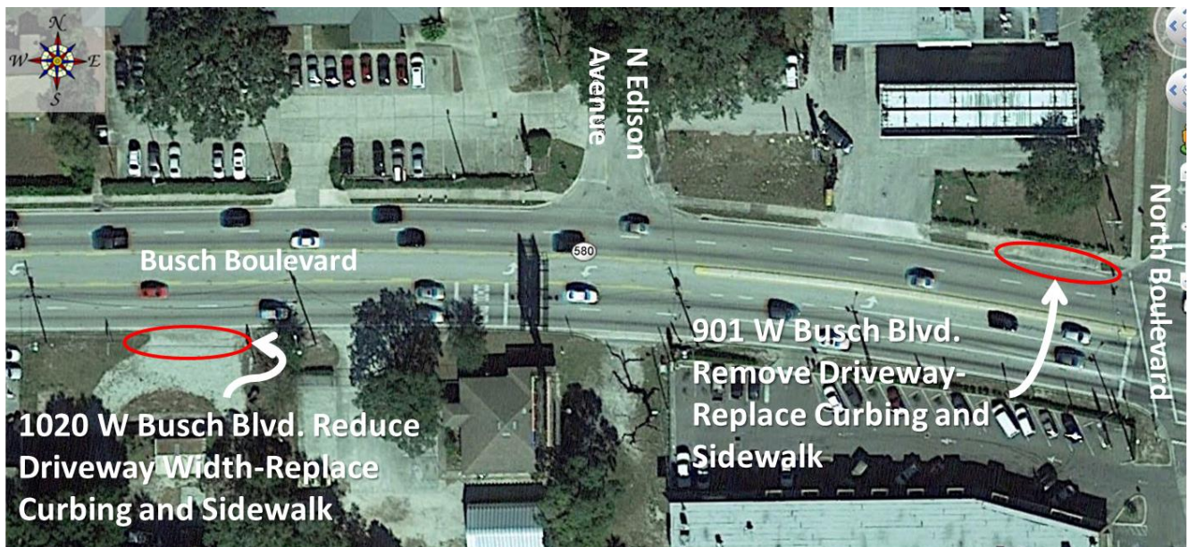
Figure 4-1: Recommended Access Modifications
