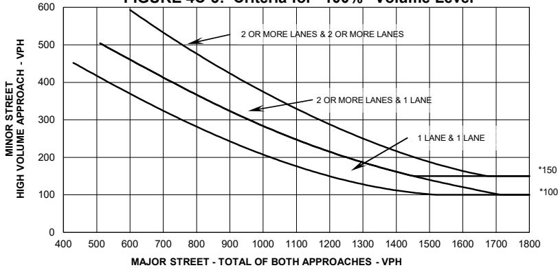
\* Note: 150 vph applies as the lower threshold volume for a minor street approach with two or more lanes and 100 vph applies as the lower threshold volume threshold for a minor street approach with one lane.
