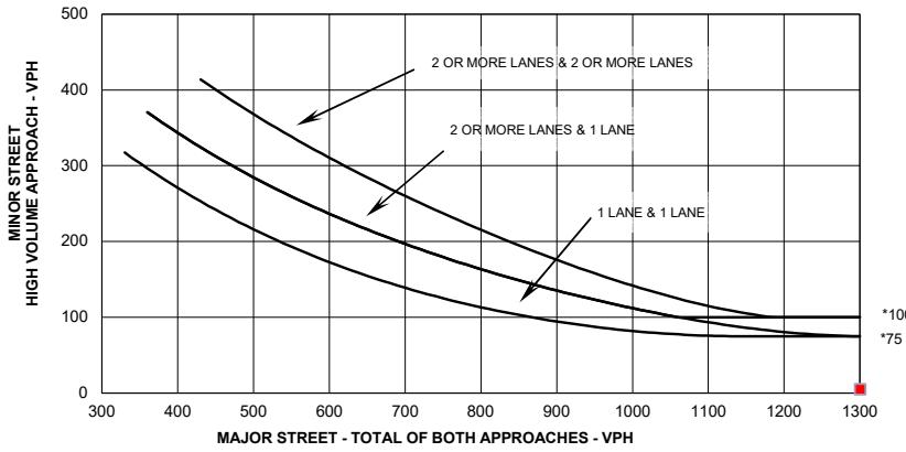
\* Note: 100 ph. applies as the lower threshold volume for a minor street approach with two or more lanes and 75 phi applies as the lower threshold volume threshold for a minor street approach with one lane.
