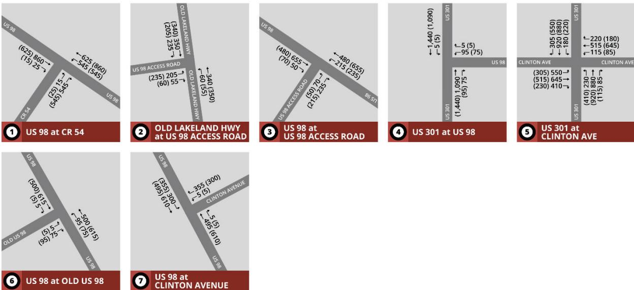
Figure 6: Design Year (2045) Build Turning Movement Volumes
