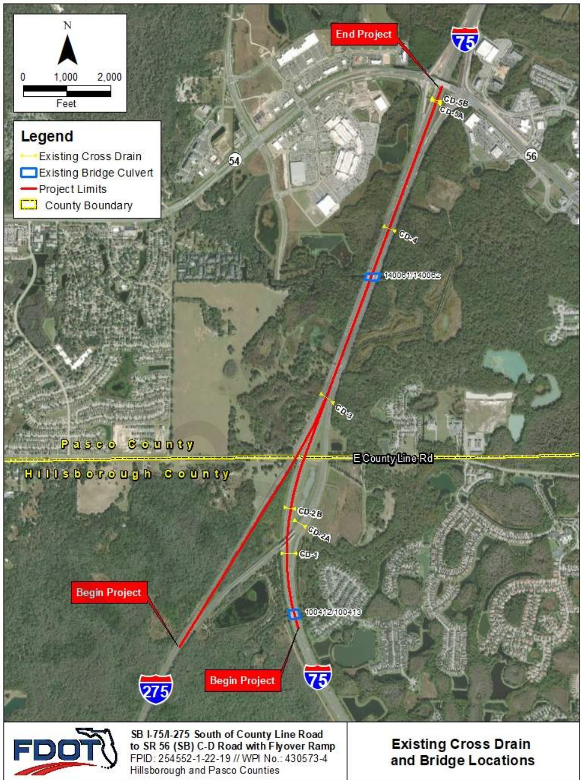
Figure B-3 Cross Drain and Bridge Map
