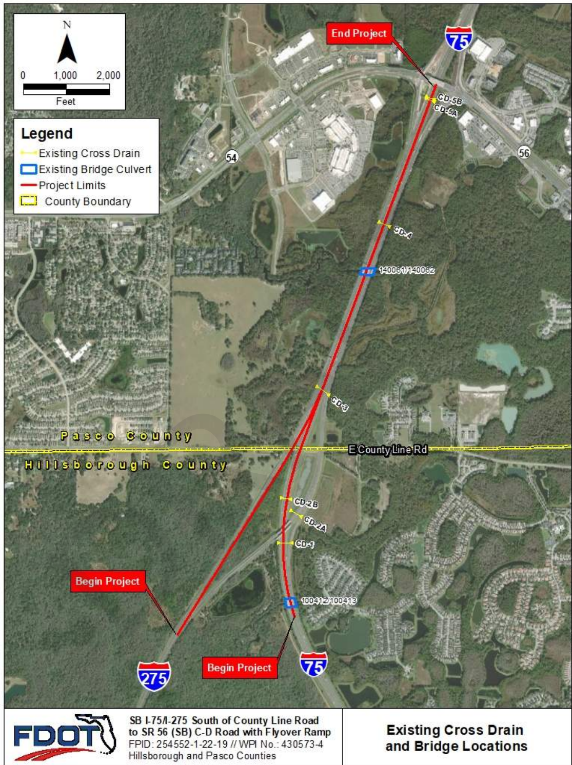
Figure B-3 Cross Drain and Bridge Map
